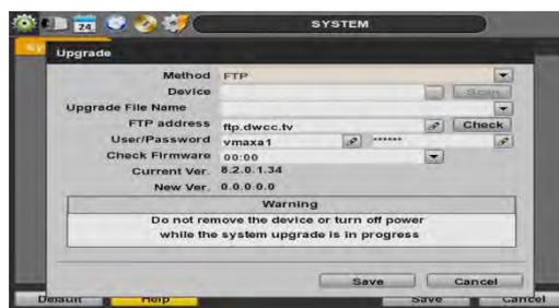
**CAUTION** It is recommended to format the HDD after firmware upgrades because the data recorded by previous firmware may cause malfunction of DVR. It is highly recommended to check all functions and menus after a firmware upgrade for proper layout and performance. If necessary, you can return system to its default settings.
