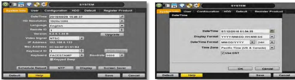
Since the clock jumps from 2:00 to 3:00, when you go to search mode, you can see there is no data in all channels for one hour due to DST.
