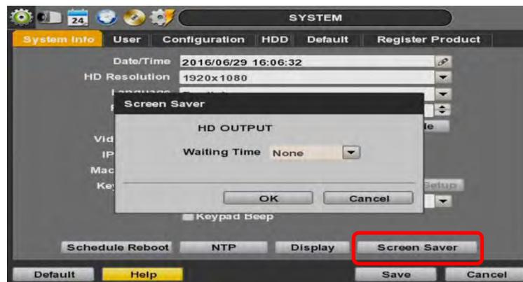
**NOTE** The Screen Saver will not work if Waiting Time is set to "NONE" or the HD output box is unchecked. Screen Saver may also be disabled during a firmware upgrade, HDD format, or data backup. The system will continue to record while the monitor is off.
